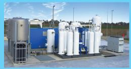
Following initial desulphurisation the PSA processes can be used to separate the mixed gases as different gases are adsorbed on different surfaces.
