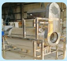
Stainless steel rotatable drum filters are used to remove the big solid particles from waste water produced by the processing industries.
